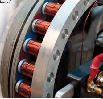
(The hybrid retrofit kit is installed in the space between the brake mechanism and the hub.)
